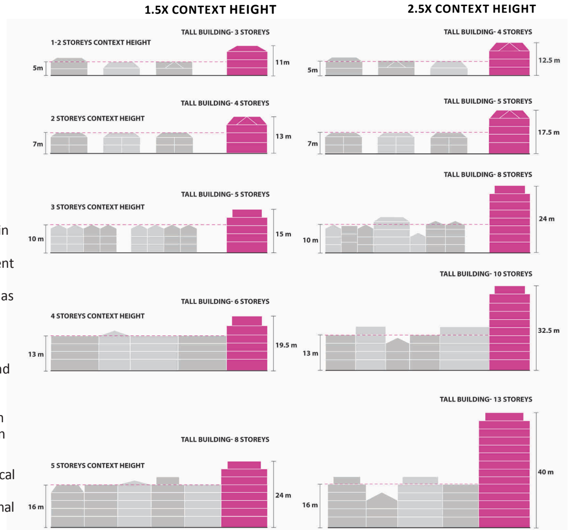
Figure 3.1: Diagram illustrating local landmarks relative to their context height (1.5x and 2.5x context height)
